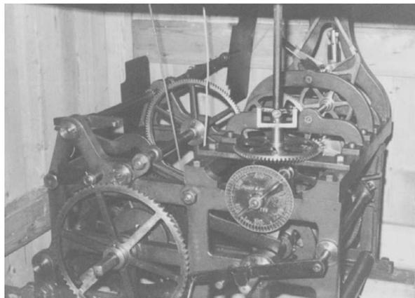
*The clock mechanism inside the tower [M20197]*
